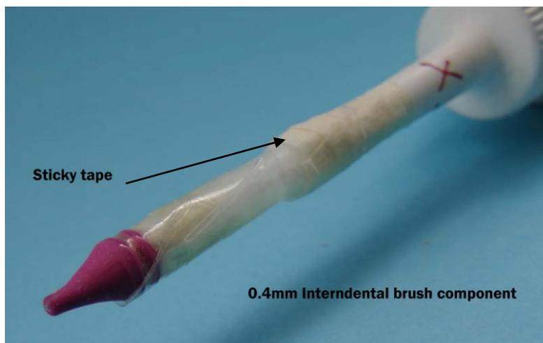
**Figure F8** – Interdental brush component fitted to nozzle
