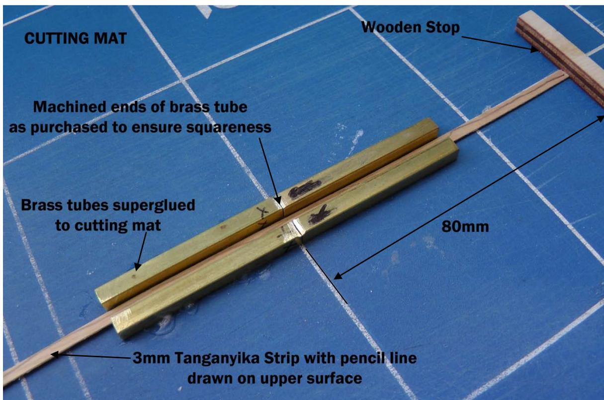
**Figure F2** – Jig for cutting plank lengths
