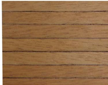
**Figure F17** – Planking demonstrating ‘caulking’ effect with all edges shaded (*test piece*)
