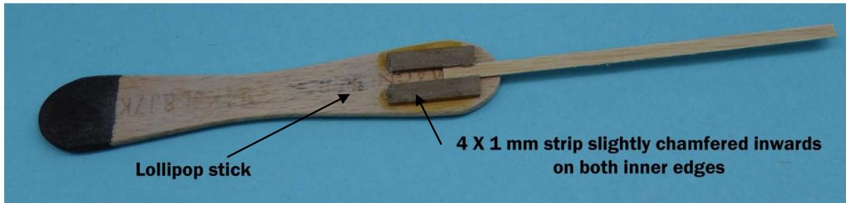
**Figure F5** – Tool for holding individual planks
