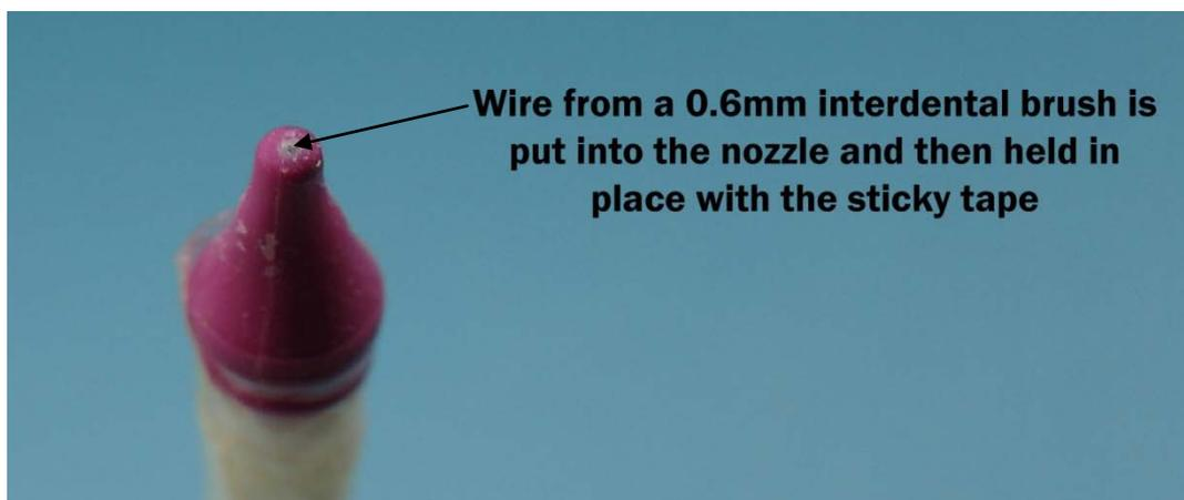
**Figure F9** – Wire threaded into nozzle
