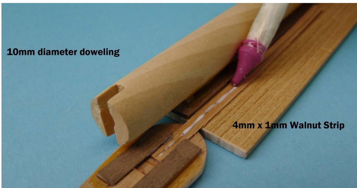
**Figure F11** – Guide for ensuring a uniform amount of glue is applied to plank
