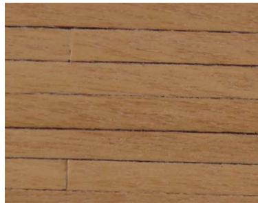
**Figure F18** – Planking demonstrating ‘caulking’ effect with one edge shaded (*test piece*)
