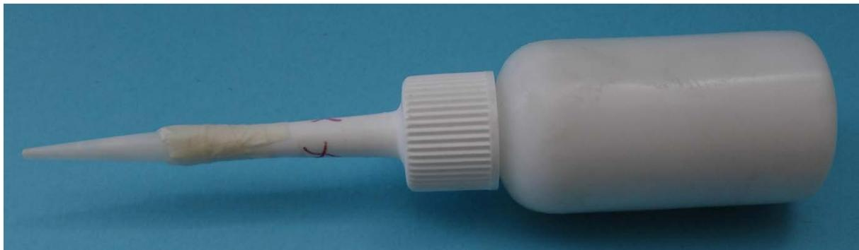
**Figure F6** – Fine nozzle fitted to glue bottle
