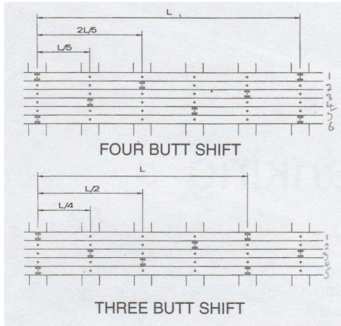
**Figure F1** – Butt system of deck planking (Julier 2005, p46)
