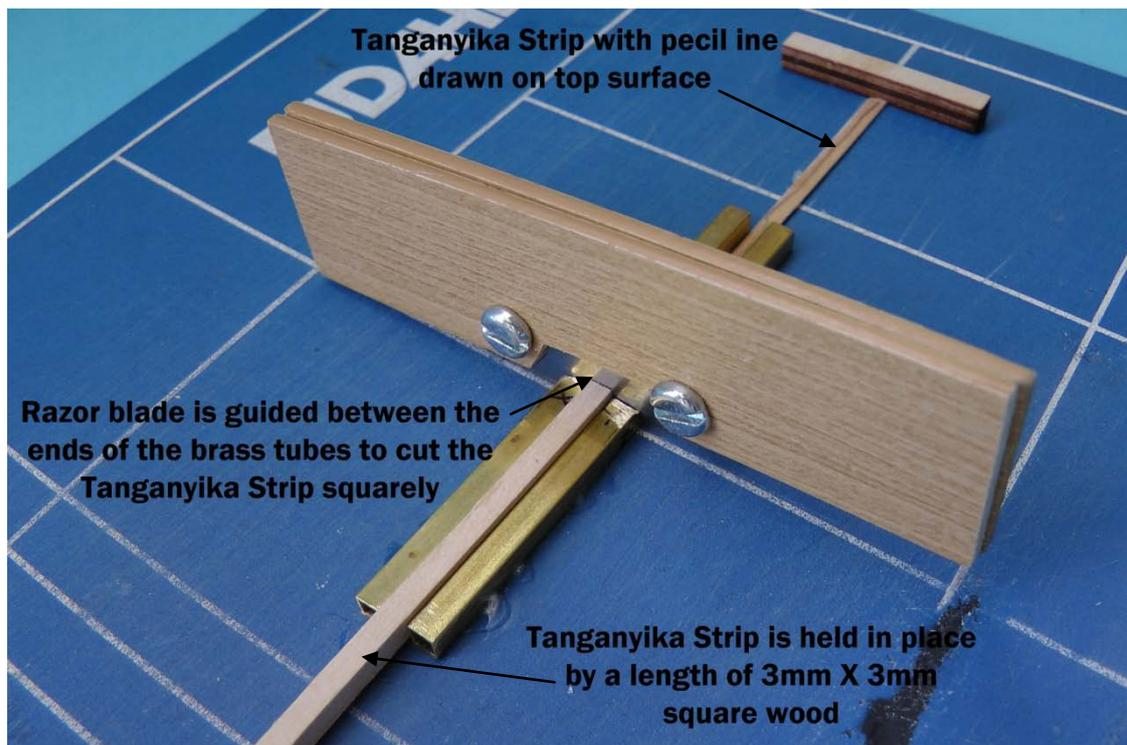
**Figure F4** – Jig used for cutting planks
