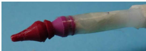
**Figure F13** - Stopper made from an “interdental brush” component part
