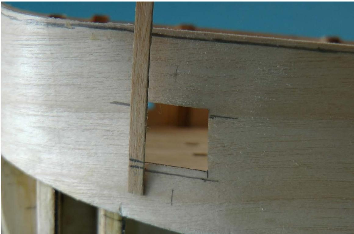
**Figure M3** - Difference at the bottom of Gun Port marked on the port side
