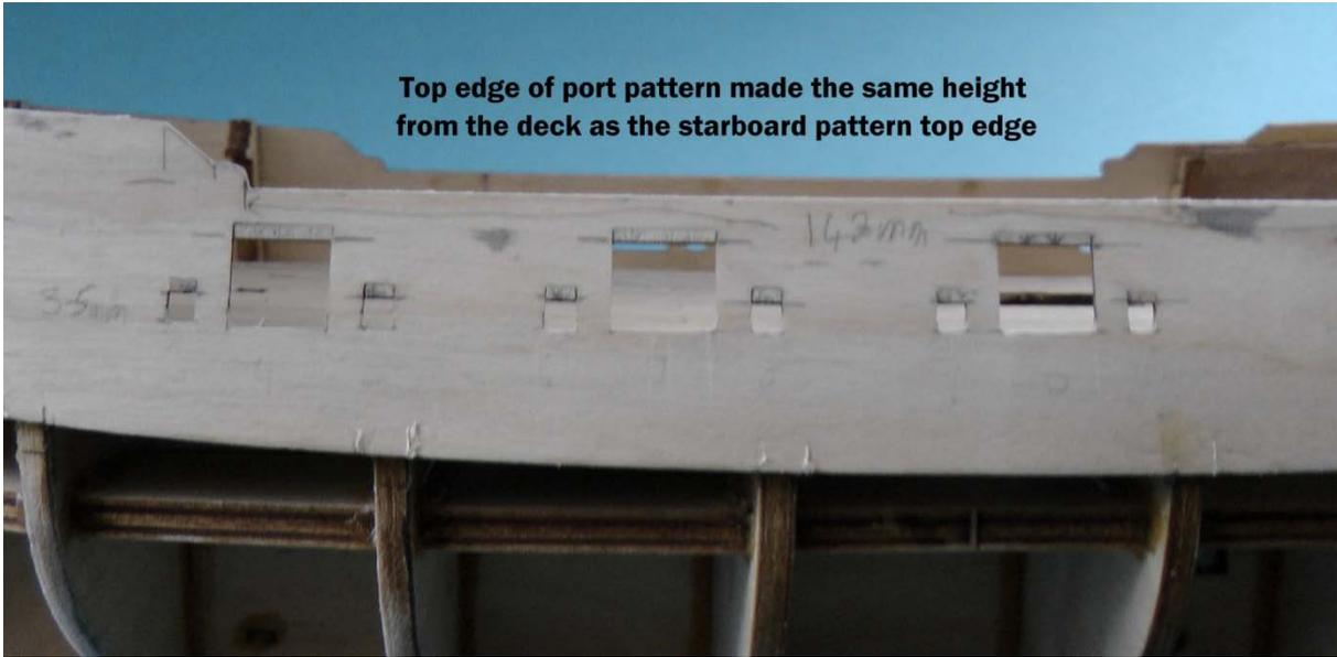
**Figure M8** - Port pattern edge made the same as the starboard edge
